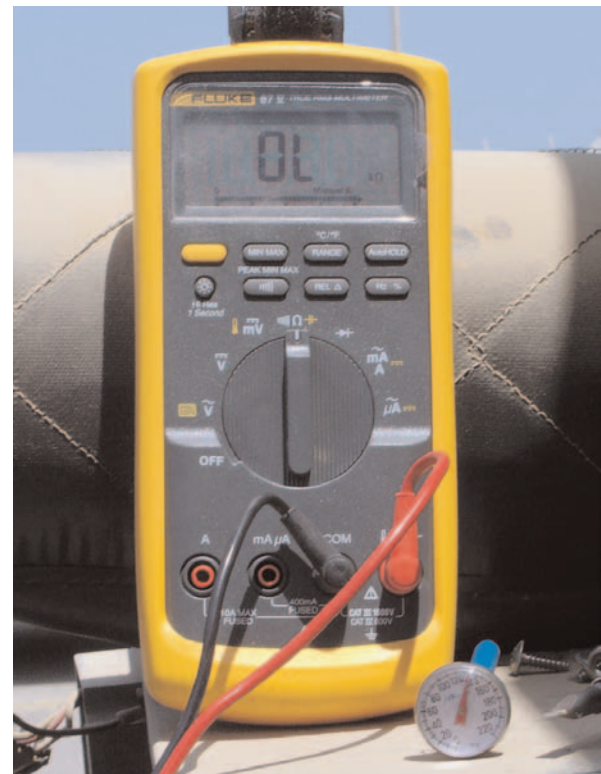
Using the Fluke 87V to check continuity in 135 °F heat.
