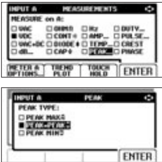
Figure 3. Easy menu selections for max-peak, min-peak or peak-peak measurements
